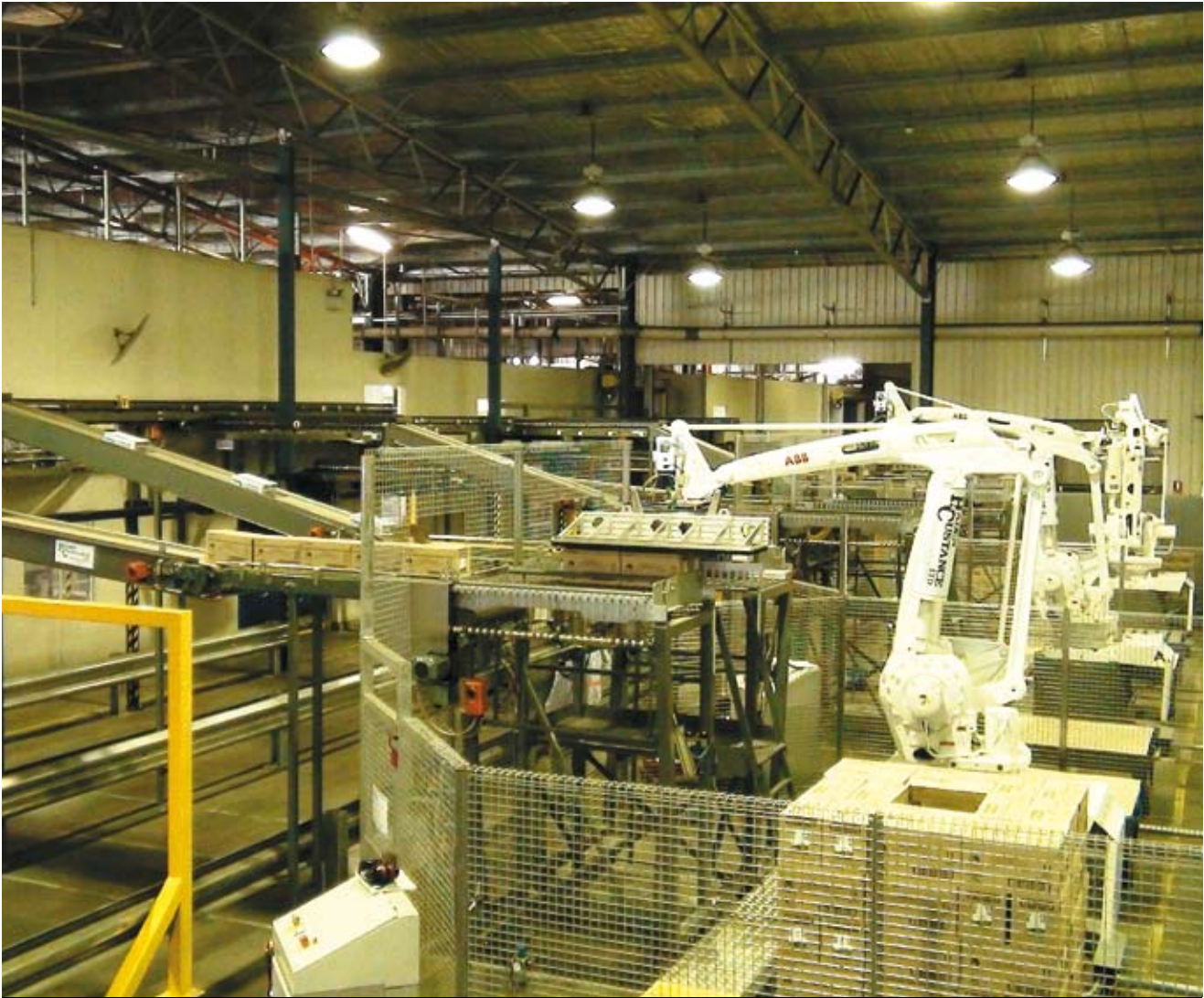
Palletising system developed and constructed for an Australian dairy manufacturer which utilised ABB 660 industrial robots
