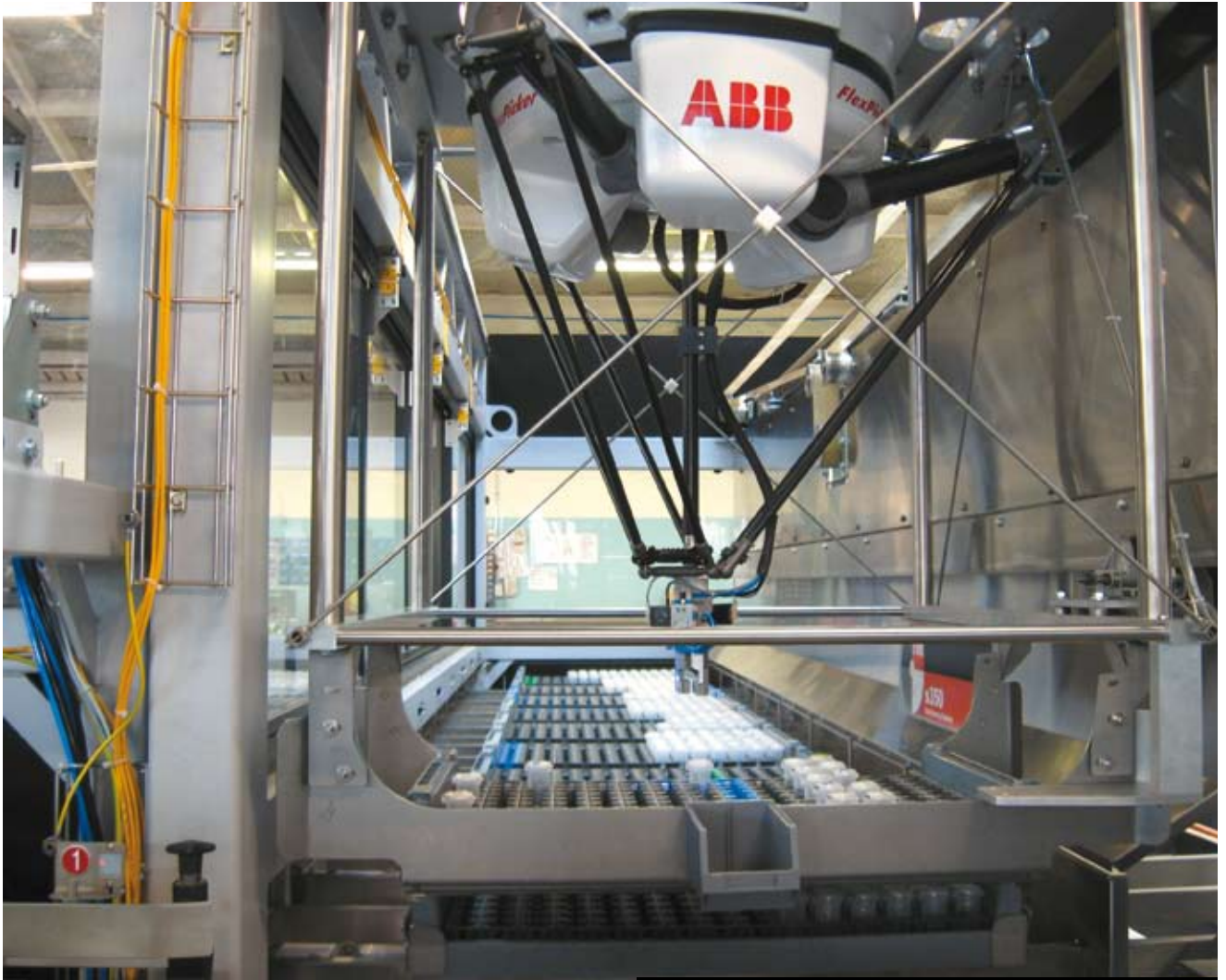
Viewed down the sample sorting chamber, the Robot takes sample vials from trays, as received, and using RFID tag information, sorts them into trays for required testing regimes. The sorter also selects and gathers samples requiring splitting
