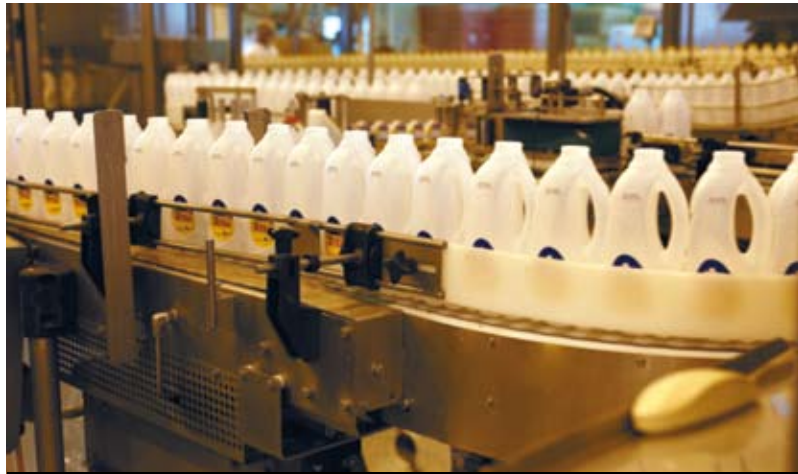
Two litre milk bottles on the production line. The site makes its own HDPE milk bottles on-site
